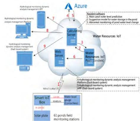
Figure 3. System communication flow chart
